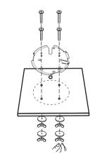
Secure the mounting bracket to the ceiling tile using pan-head screws, washers, and wing nuts, as shown on the left.
