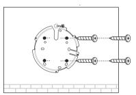
Secure the mounting bracket to the wall by driving the self-tapping screws into the anchors. Make sure that the shoulders of the mounting bracket are on the outside.
