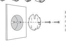
Route the cables through the square cable hole on the mounting bracket, and secure the mounting bracket to the junction box using screws. Then follow Step 4 and Step 5 of Option 2 to complete the installation.
