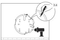
If your Ethernet cable feeds through the wall, position the mounting bracket below the cable hole. Mark positions for the screw holes and drill 6 mm (15/64 in) diameter holes at the marked positions.
