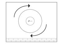
Attach the EAP to the mounting bracket by rotating it until it locks into place, as shown on the left.
